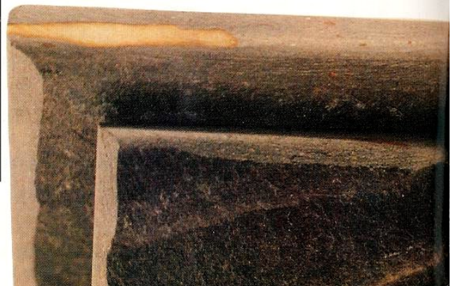
Some of the problems which can be encountered with slate. The picture at the top shows what happens when calcite inclusions burst as a result of mild acid attack. Above, the slate is showing signs of delamination as a result of acid immersion testing. And the slate below shows an area of discoloration during a wet/dry cycle of testing.
