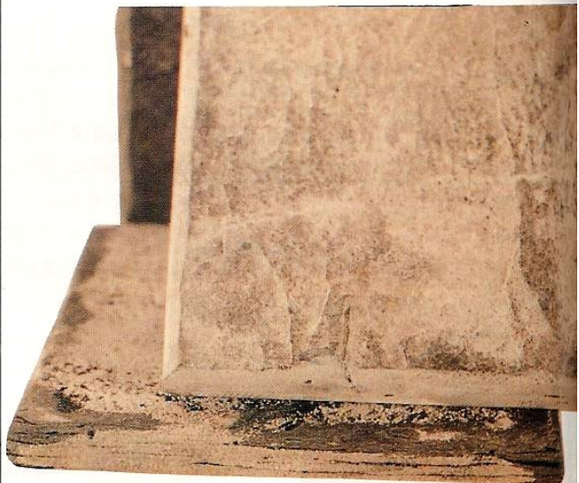
Some of the problems which can be encountered with slate. The picture at the top shows what happens when calcite inclusions burst as a result of mild acid attack. Above, the slate is showing signs of delamination as a result of acid immersion testing. And the slate below shows an area of discoloration during a wet/dry cycle of testing.
