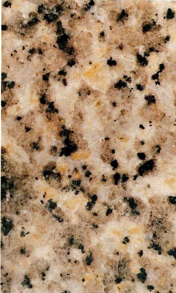
Below: Fig 2. Discolouration from white to orange of feldspar crystals at the polished surface of a granite. Magnification: x 2.
