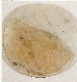
Left: Fig 4. Dark patches in a travertine floor due to different concentrations of dirt in unfilled voids. Above. Fig 5. Discolouration of Carrara marble.
